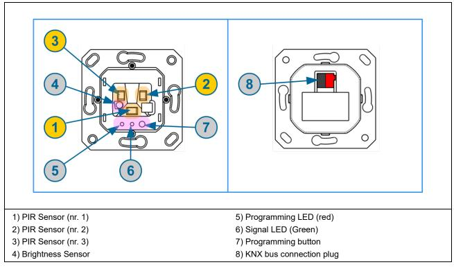
The device is equipped with a programming pushbutton and a programming LED, a signal LED, three PIR infrared sensors and a brightness sensor.
